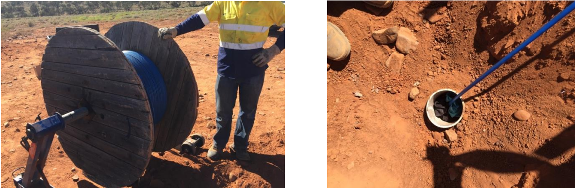
Figure 1 Left: DAS cable on its reel showing the ease of deployment – no need for special winches. Right: A DAS cable inserted in MSDP02 borehole. The rugs in the hole are to protect the hole from "air-blast" – a wave induced by air-wave produced by the source.
